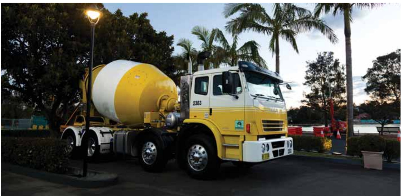
A concrete delivery truck, also known as a concrete agitator
