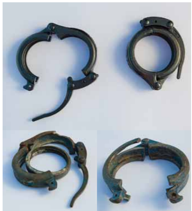
New and damaged pipe clamps
